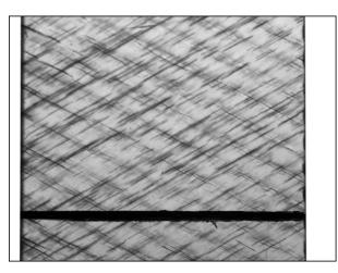
*CrackDect* works only on images similar to the one above, where cracks appear dark on a bright background. The cracks must be straight, since the currently implemented algorithms work with masks and filters to extract cracks in a specific direction. Therefore, it is possible to only detect one kind of cracks and ignore cracks in other directions.
