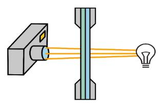
This technique results in a bright image of the specimen with dark crack like this.
