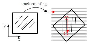
5. Crack Density: The crack density is computed from the detected cracks with
