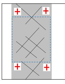
The red crosses are used to correct the shift and distortion of the image while the blue dotted rectangle would mark the usable region of interest for the crack detection.
